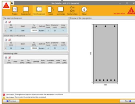
**Gambar 4.** Permodelan Elemen Balok Pada SIKA CarboDur
